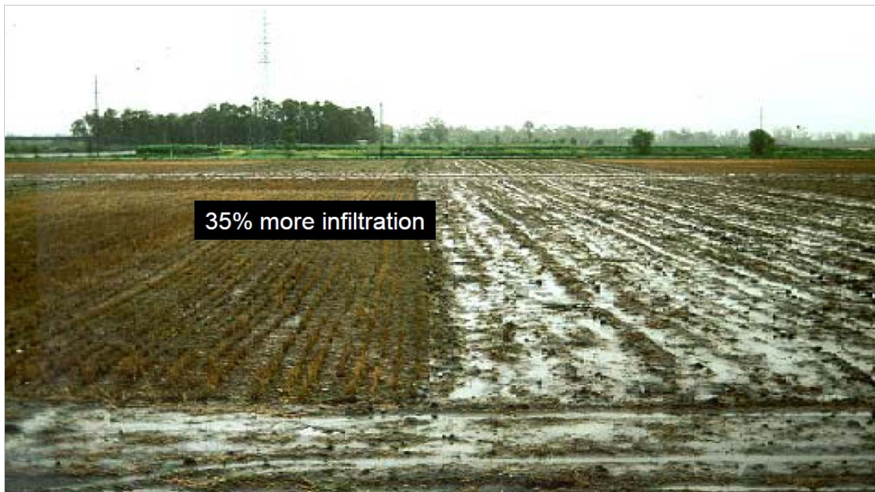
Figure 24b: A dramatic demonstration of the impact of soil compaction. The soil of an experimental plot (Italy) has been subjected to heavier loads on the right-hand side of the image than on the left-hand side. The compacted structure of the soil on the right has resulted in a reduced infiltration capacity of the soil, leading to surface ponding and waterlogging. © Ezio Rusco
