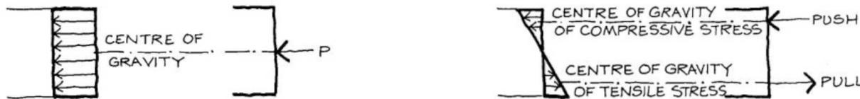
Because the push equals the pull, the combined force can only be an axial force. But this force must act at the centre of gravity of the combined stress distribution.
