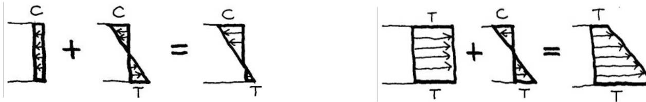
The axial stress distribution can be thought of as an axial force acting at the centre of gravity of the axial stress distribution and the bending stress distribution can be thought of as a pair of *push-pull forces* acting at the centres of gravity of the tensile and compressive parts of the bending stress distribution.
