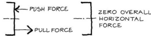
Secondly, from moment equilibrium, the size of the bending moment is equal the size of the push force times the lever arm, or the size of the pull force times the lever arm.
