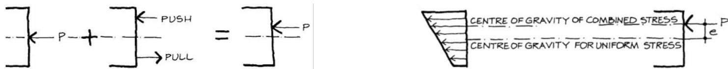
The effect of the moment is to ‘move’ the axial force by a distance,  $e$ , from the center of gravity for uniform axial stress. This distance  $e$  is called **eccentricity**.
