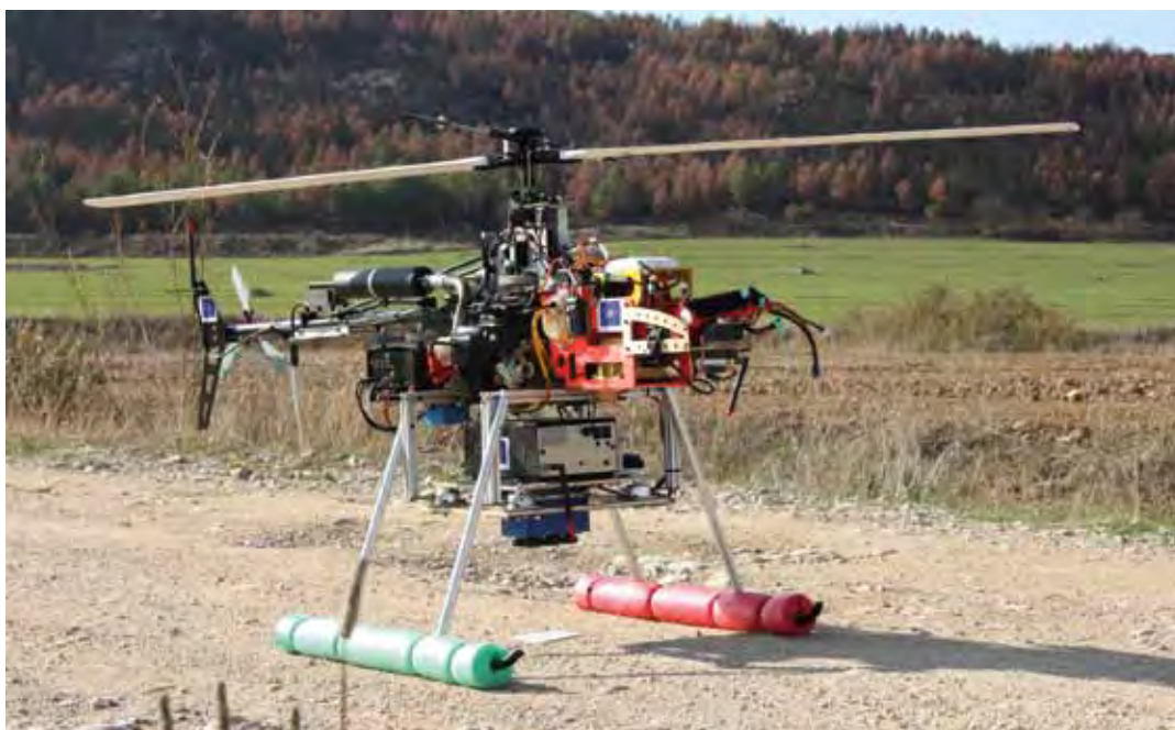
AG_UAS is using airborne sensors on drones to identify crop irrigation needs in Navarra
